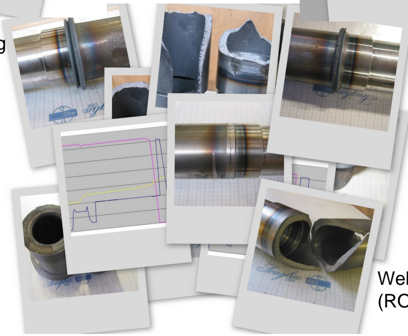
Welding of cast irons with using welded inserts (ISQ)
